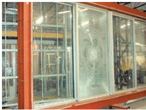
Large missile hurricane impact tested HPX Slider
