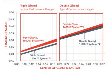
Each infill option offers two levels of performance ranges. These depend on pressure plate choice (aluminum or fiberglass) and system type. The fiberglass pressure plate option not only enhances thermal performance, but also improves condensation resistance.
