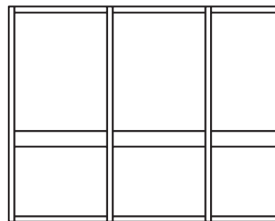
RAILING MOUNTED BETWEEN MULLIONS
